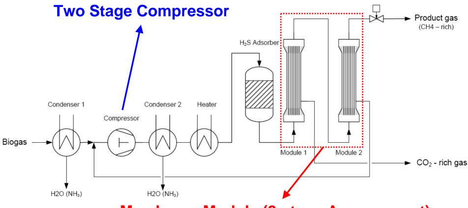
Membrane Module (2-stage Arrangement)
