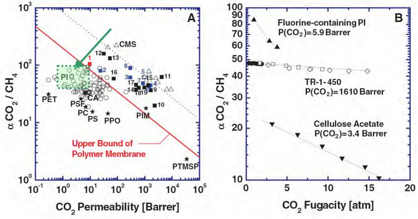
Relation between CO2 permeability and CO2/CH4 selectivity of TR polymers (PI derived polymers with intrinsic cavities) From [H. B. Park et al., Science 318, 254 -258 (2007)] Reprinted with permission of AAAS
